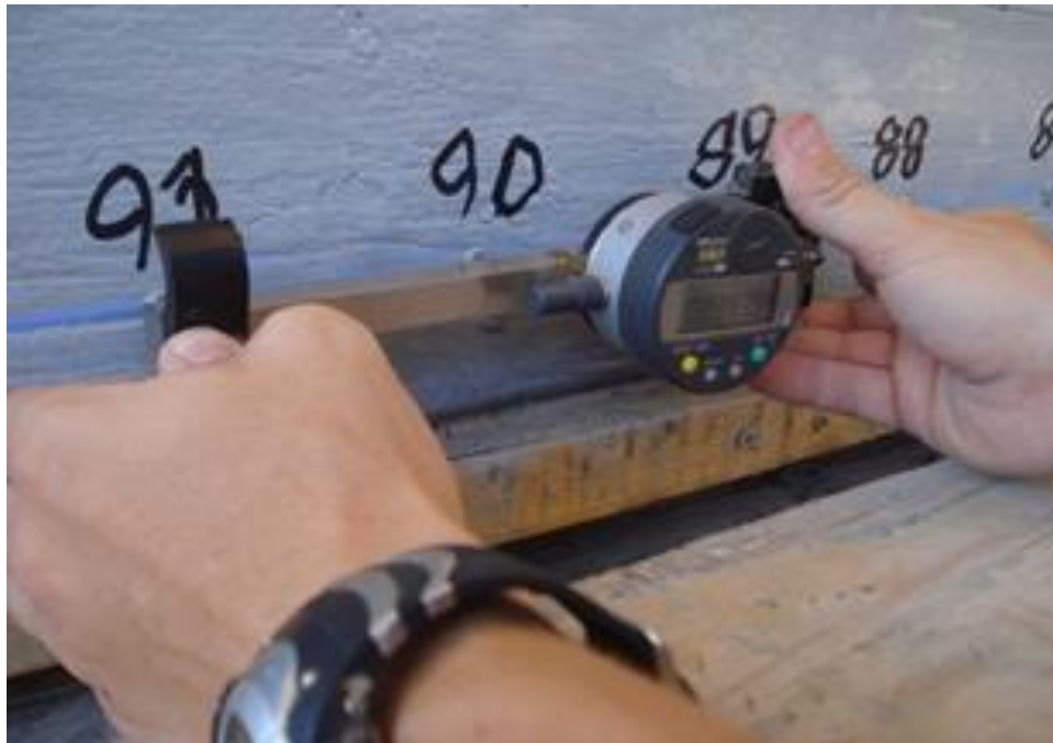
Figure 2-3. DEMEC measurements (Photo by author).
